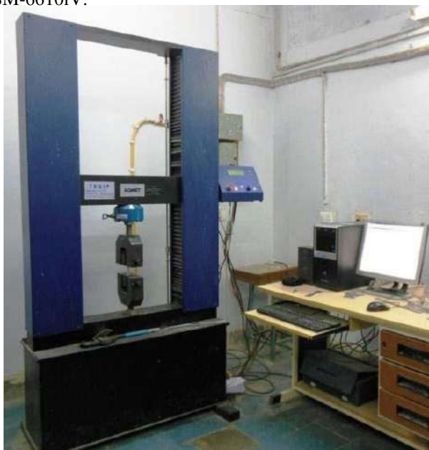
Fig 1. Specimen loaded on Universal Testing Machine
