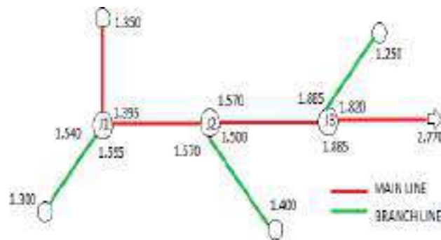
Fig - 2: Final solution with invert depths
